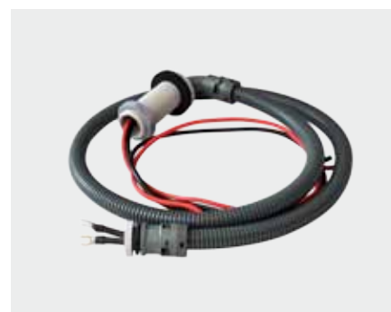
KT1-10 707210 1-EXIT ROOF DUCT provided with cable sheath L=1m and 2 x 6mm 2 L=2m cables.
