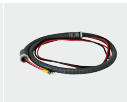
KT5-C10 707051 KIT FOR "KT5" provided with cable sheath L=1m and 2 x 6 mm 2 2m long cables. Provided with PG11 fittings and terminals for photovoltaic module connection.
